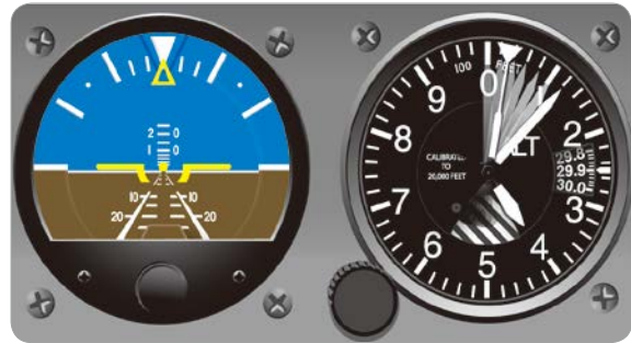
[그림 3-49] Using the altimeter for pitch interpretation, a high altitude means a nose-high pitch attitude
