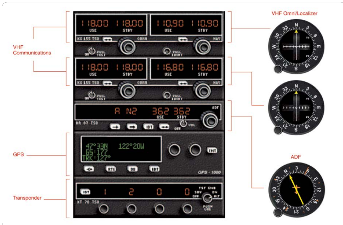
[그림 5-1] Typical navigation/communication installation
