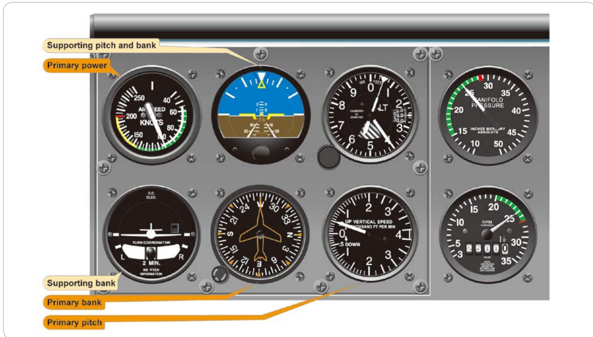
[그림 3-69] Stabilized climb at constant rate
