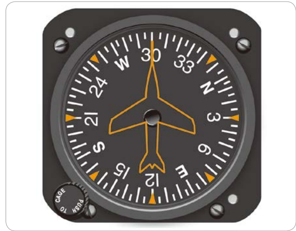
[그림 3-28] The heading indicator is not north-seeking, but must be set to agree with the magnetic compass
