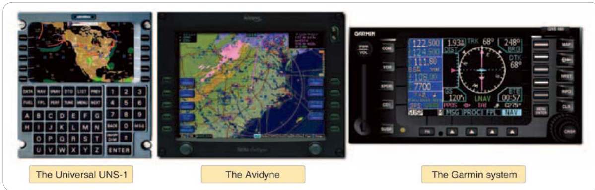
[그림 2-38] Typical display and control unit(s) in general aviation
