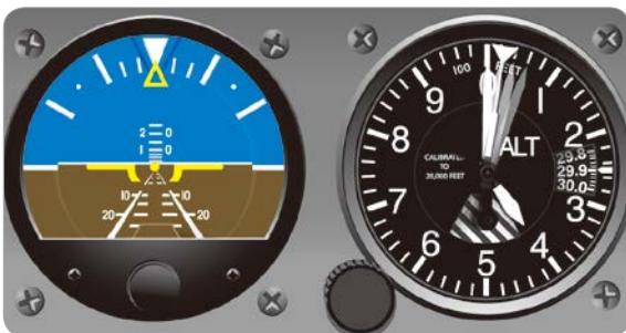
[그림 3-52] Pitch correction, less than 100 feet-1/2 bar low to correct altitude error
