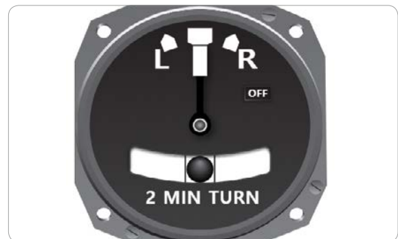
[그림 2-95] Turn indicators rely on controlled precession for their operation
